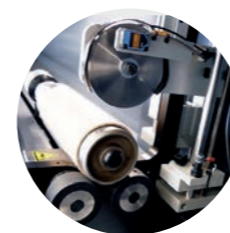
STEEL ANVIL FOR PRECISION CC160/200 is born with a steel anvil for high precision cutting of cores. Other anvils are available for different core sizes and wall thicknesses.
