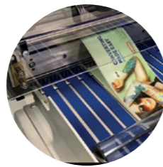
HIGH SPEED SHEETER This high-speed sheeter cuts sheets with a speed of up to 30 m/minute or up to 14,000 sheets/hour.
